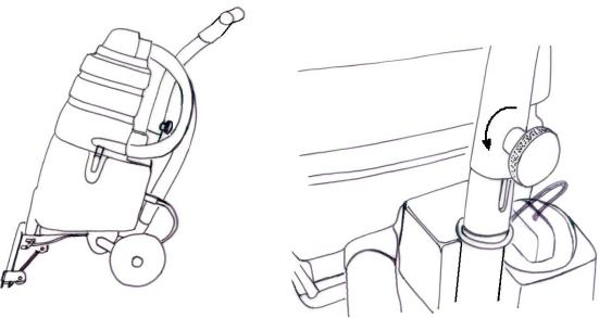
2. Fill in the lower tank (solution tank) with cold or warm water, through the filling hole, adding a 5% of not-foaming detergent (1/2 liter each 10 liters). Higher concentrations can be used in case of particularly dirty surfaces.
