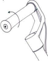
3. To clean carpets, rotate the lever on the vacuum head towards the right side. To clean hard floors, rotate it towards the left side.
