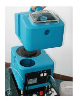
6. Put some fresh or warm water into the solution tank, through the circular hole, adding the product T-FOAM, in the dilution rate: 1 part of chemical to 4 parts of water (we suggest you should put not more than 2 litres chemical and 8 litres water).
