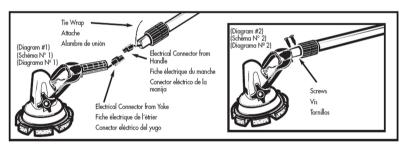
To operate Motorscrubber using the rechargeable battery, connect the electrical plug from the battery with the electrical plug in the red grip handle (Diagram #3)
