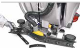
Rubber blades replacement or rotation are carried out in few seconds without any tools
