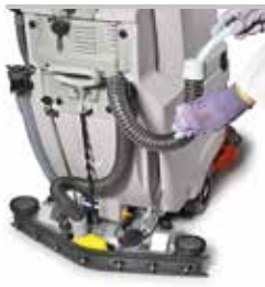
To ensure a perfect drying, the suction hose and the squeegee rubber blades must be cleaned at the end of any cleaning operation. The squeegee can be lifted to quickly clean the rubber blades
