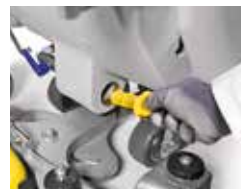
Solution filter cleaning
